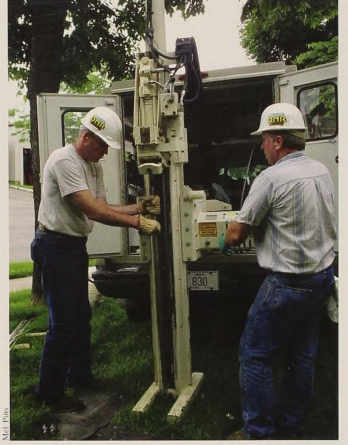
DNR staff use state-of-the-art equipment to sample and test sites for possible contamination.
