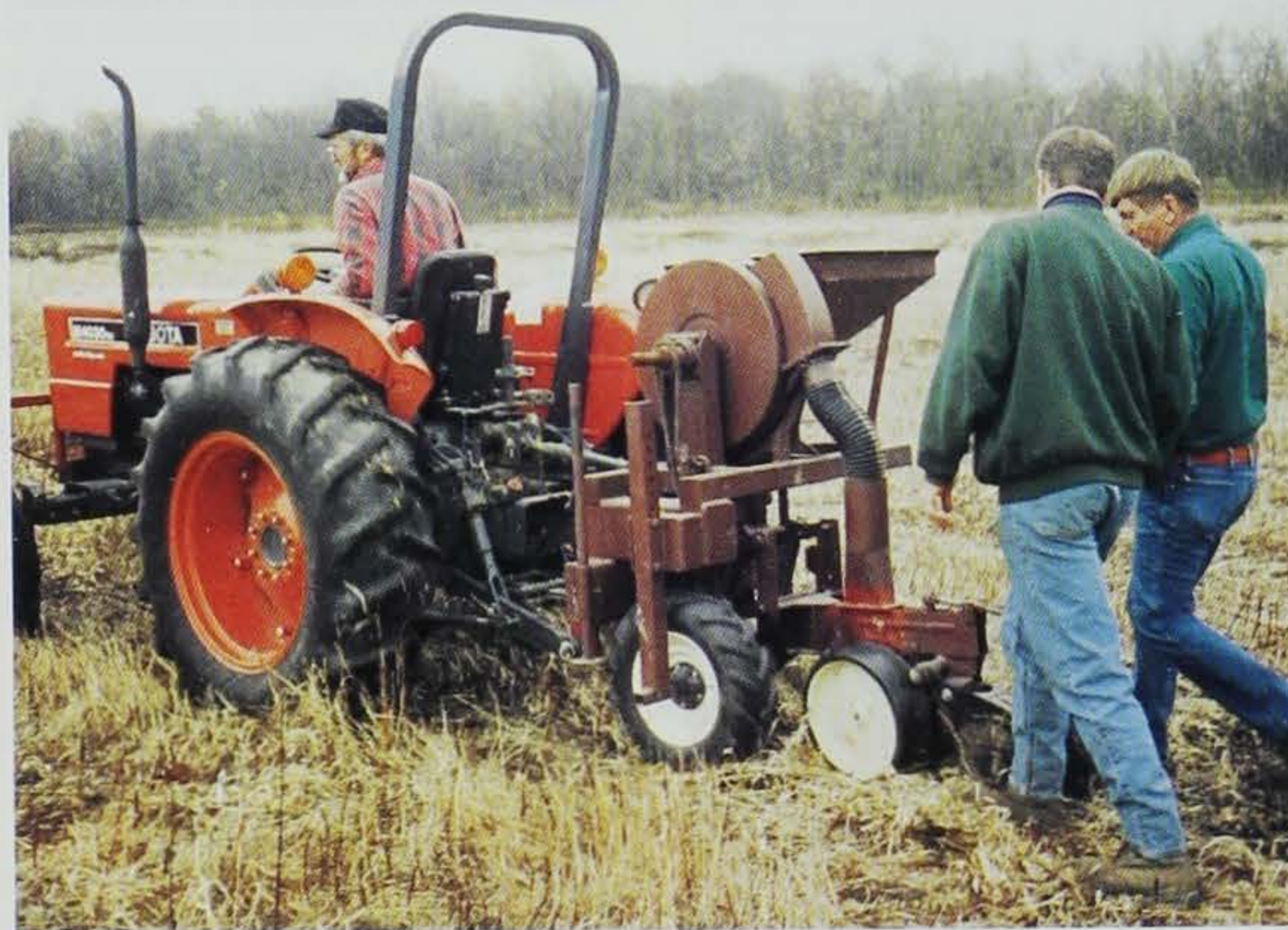
This prototype direct seeding machine allows a single operator to plant up to 20 acres per day. It is capable of planting walnuts and acorns as close as 6 inches apart in the row while traveling 2-1/2 m.p.h..
