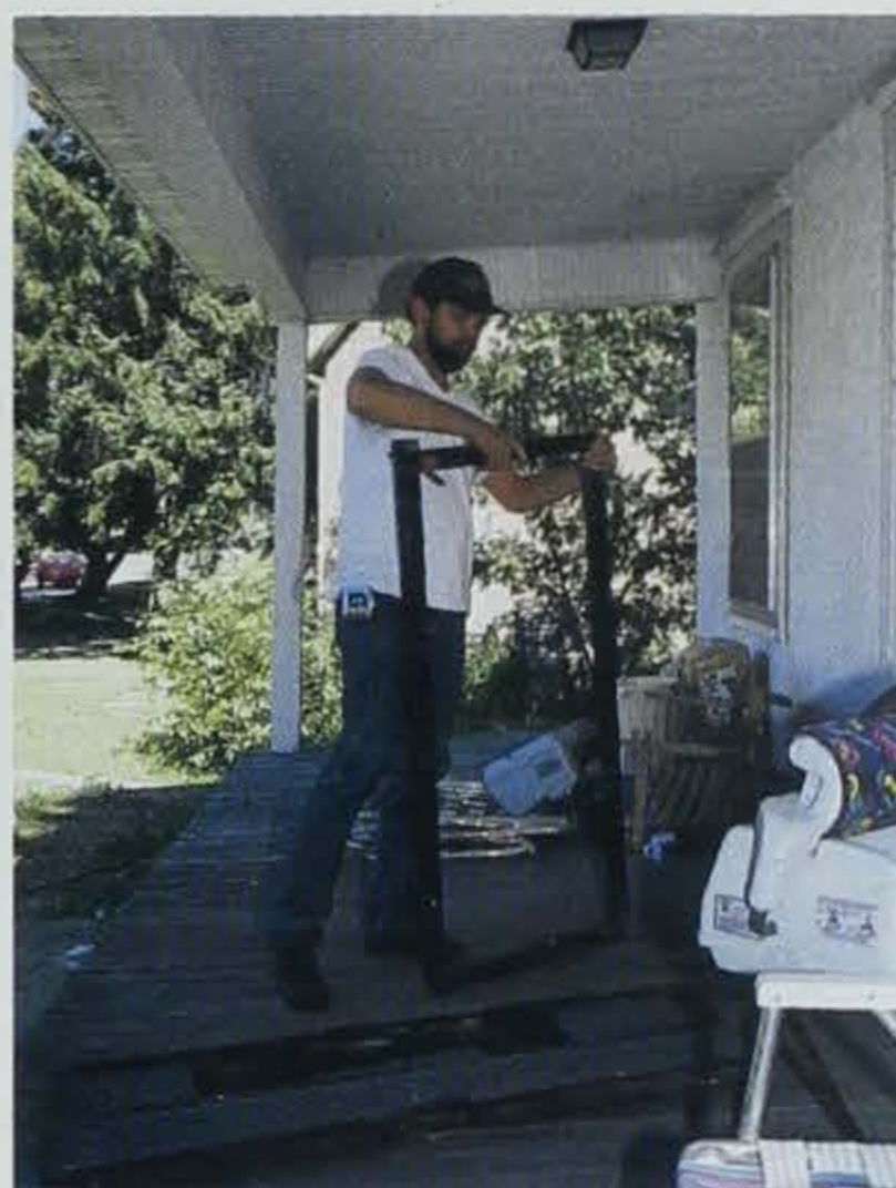
MICA has championed the use and evaluation of the blower door, which tests a home's airtightness.
