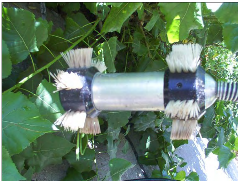
Figure 244. Snake camera used to inspect subdrains
