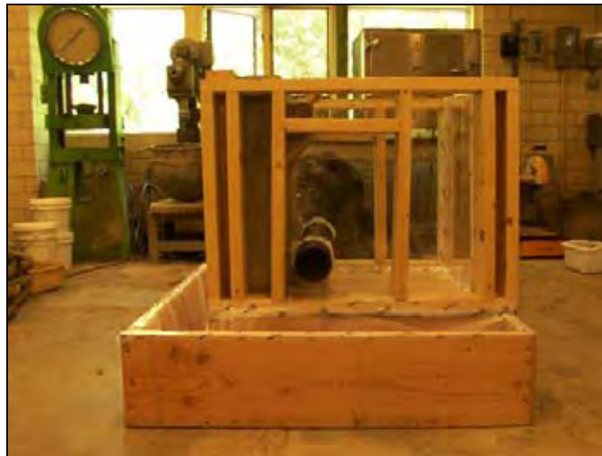
Figure 352. Water Management Bridge approach Model
