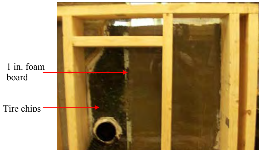
Figure 388. Drainage detail for Test 9
