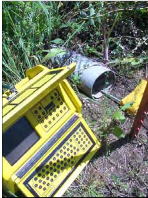
Figure 245. Control of snake camera
