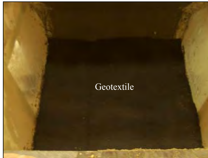
Figure 376. Placing backfill reinforcement
