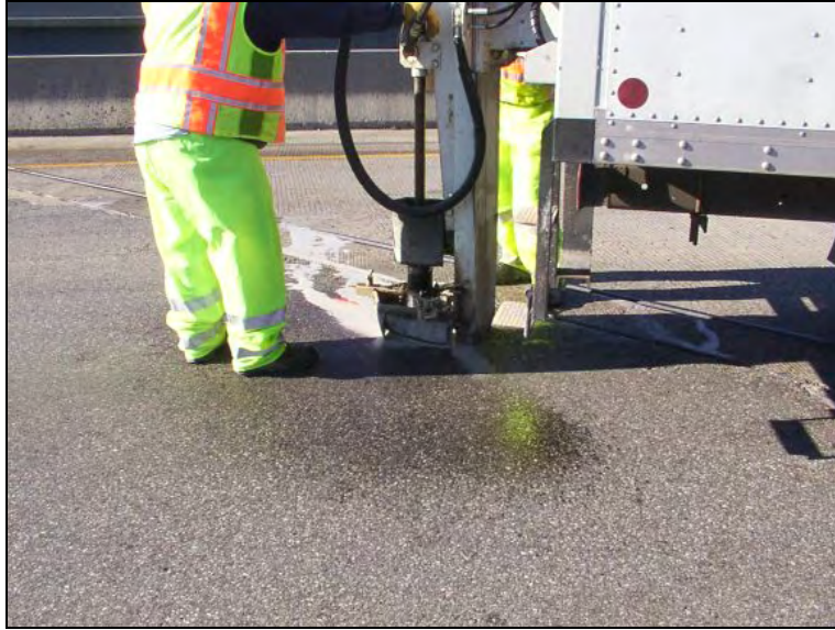
Figure 313. Coring at bridge approach (NBL)
