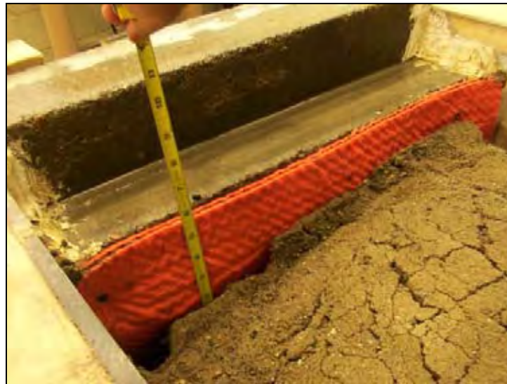
Figure 383. Void developed under the approach slab
