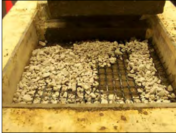
Figure 362. Placing special backfill over geogrid
