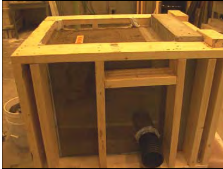
Figure 365. Granular backfill placed behind the abutment
