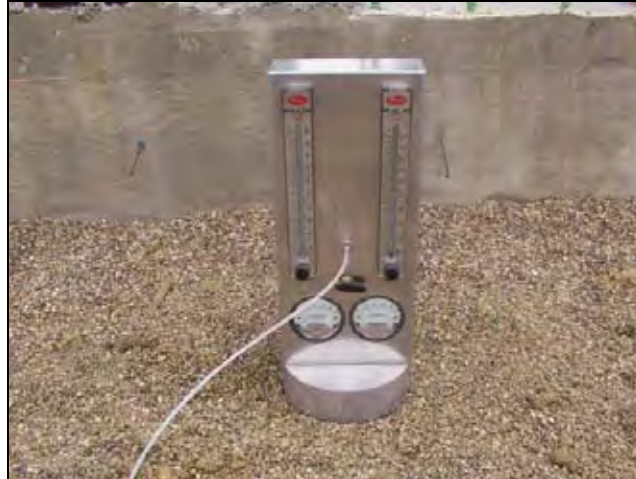
Figure 188. Air Permeability Test performed at porous backfill
