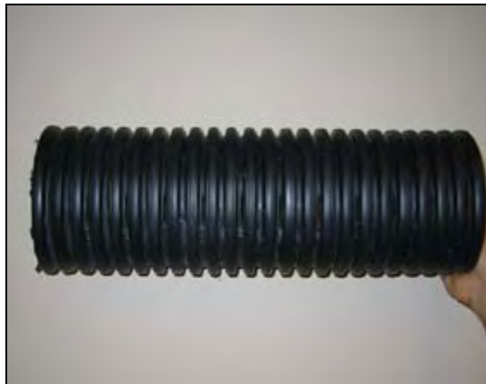
(a) Perforated drainage pipe
