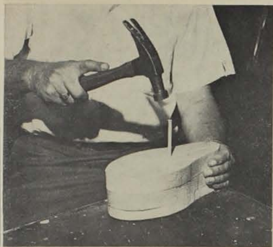
3. Three layers are then drilled and pinned together with two wooden dowels. Note: do not glue together at this point.
