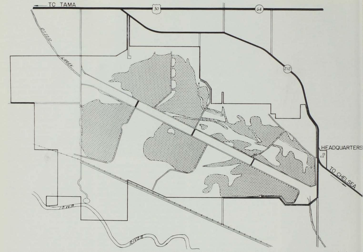
The above map of lowa's newest marsh locates the relocated channel of Otter Creek, the steel piling dams, the seven individual marshes, Unit Management headquarters and the boat ramp on the lowa River.
