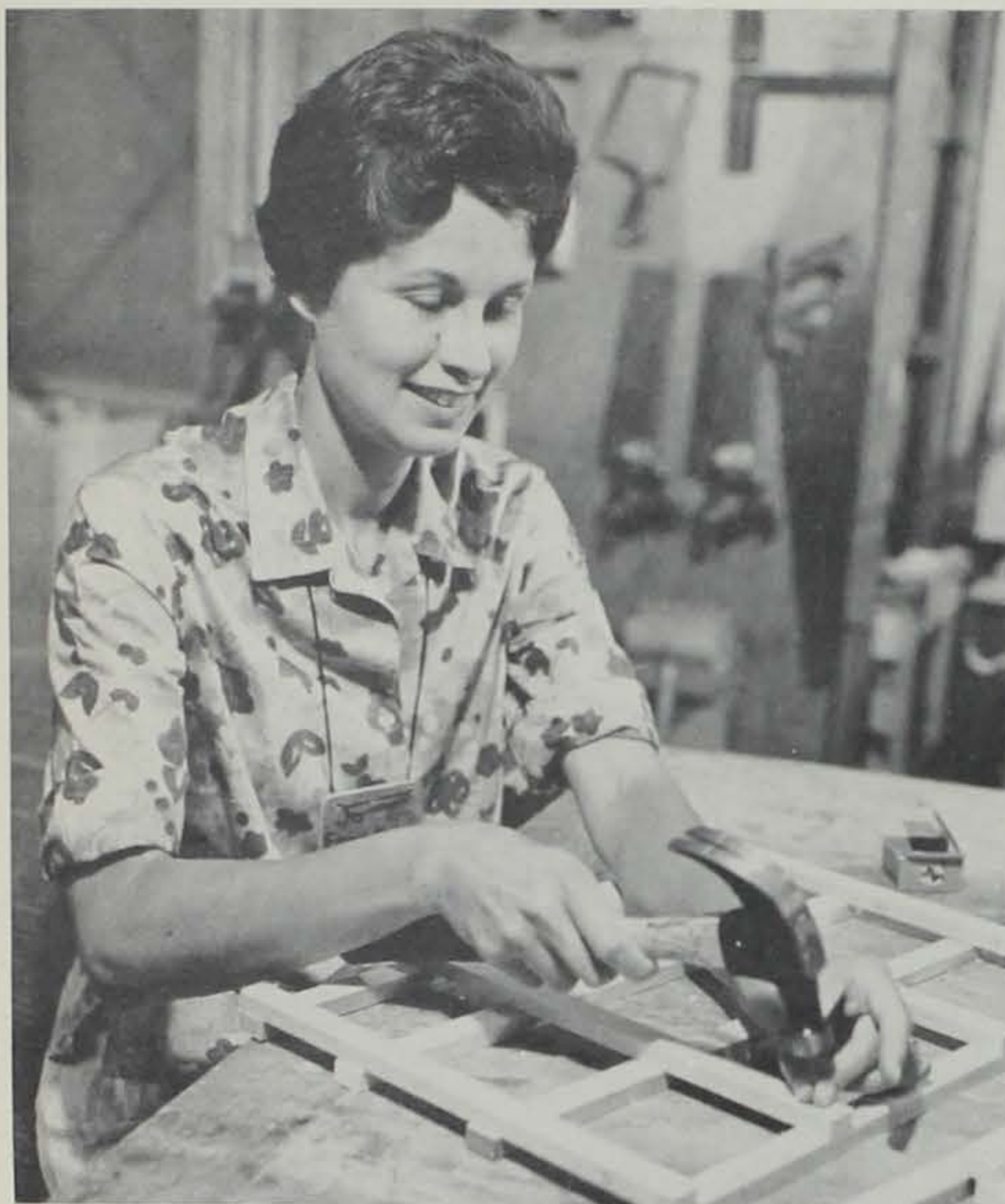
Square the corners of the press, and glue each strip before nailing.
