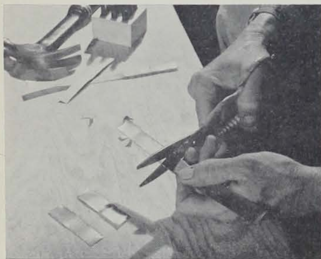
The light aluminum is easily cut with a kitchen shears. Non-deteriorating metals such as aluminum, copper, and zinc are recommended.
