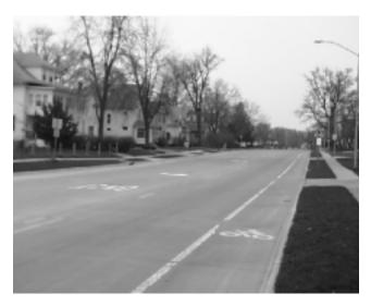
Figure 8 Three-Lane Cross Section with Bike Lanes
