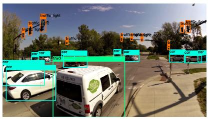
Sample vehicle detection results obtained from videos recorded at 13th St. and Stange Rd. intersection in Ames, Iowa
