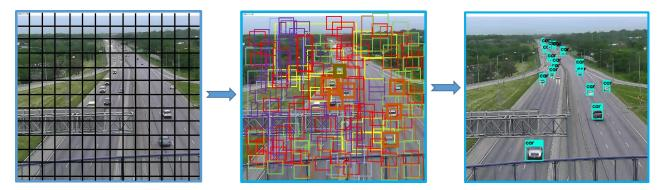
Figure 2. Confidence score prediction of bounding boxes by YOLO with colors and bounding box widths indicating confidence score probabilities
