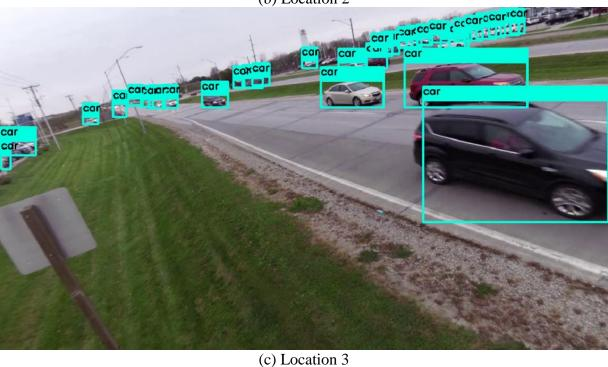
Figure 5. Sample vehicle detection results obtained from videos recorded in locations given in Table 1
