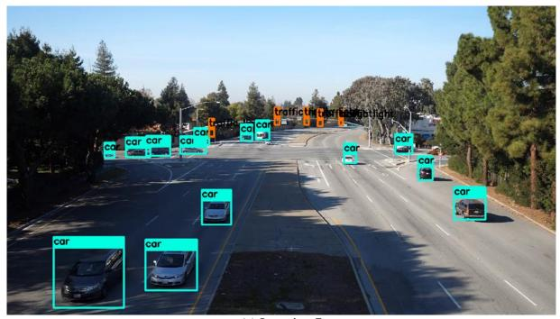
Figure 6. Sample vehicle detection results obtained from videos recorded in locations given in Table 2
