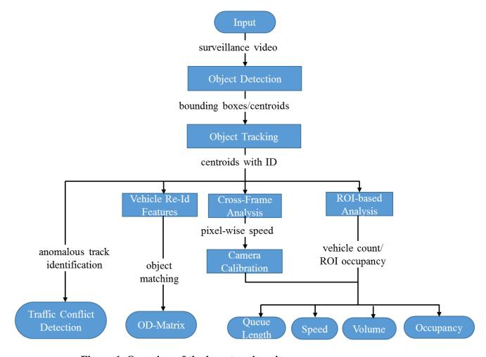
Figure 1. Overview of the key steps in using cameras as a sensor
