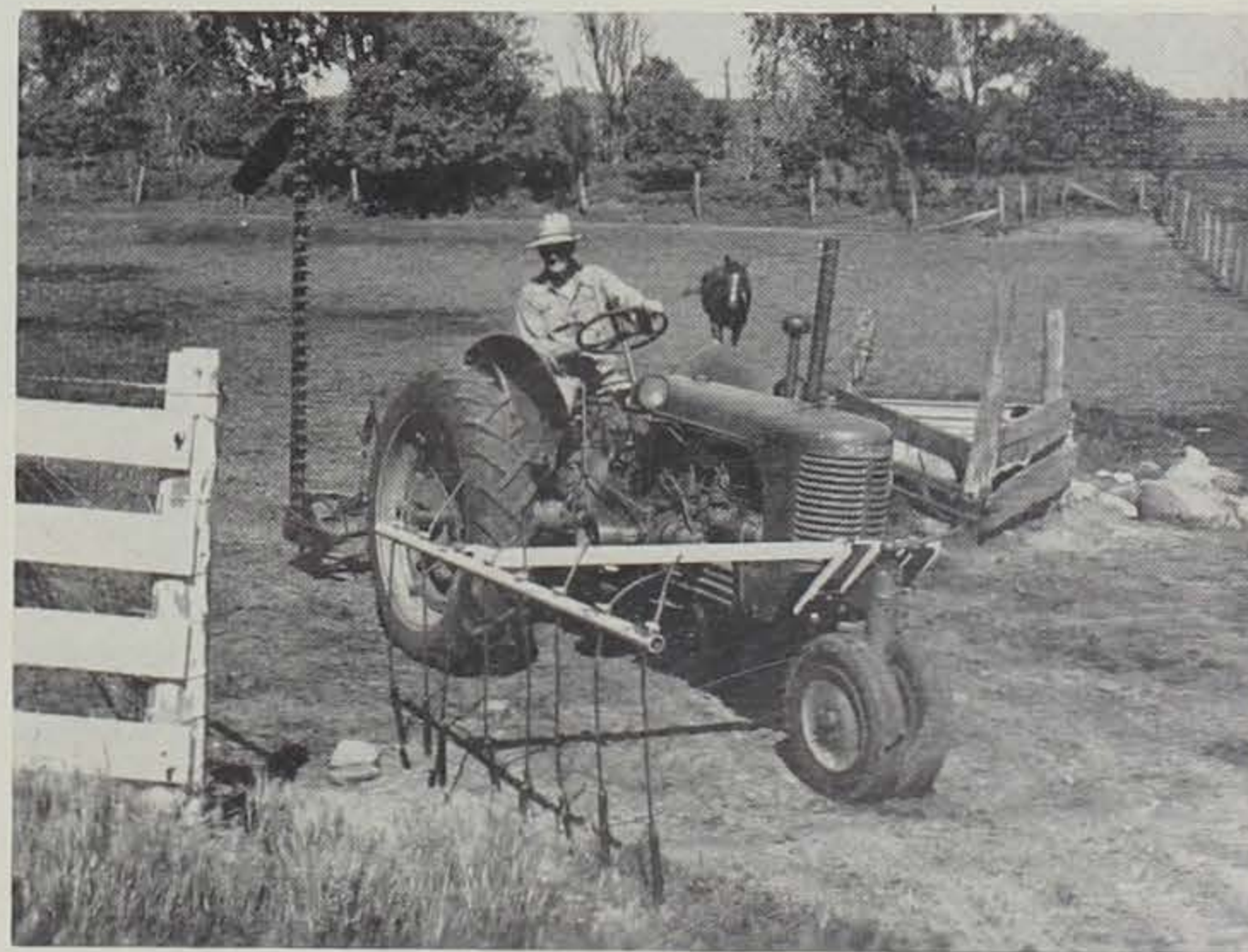
The flushing bar is folded forward for movement through a gate.
