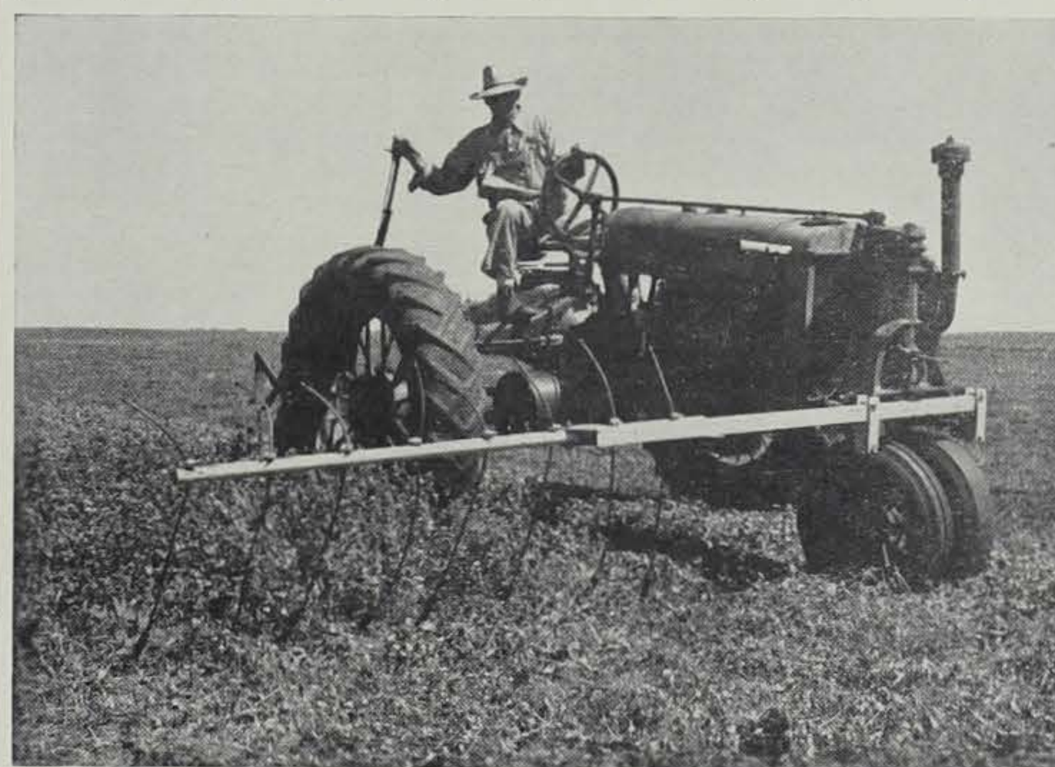
Flushing bar in action, the cables have just broken through the alfalfa. Cutter bar is twelve feet behind.
