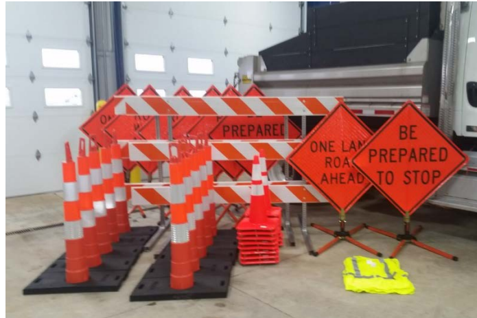
Figure 1. Work zone sign package
