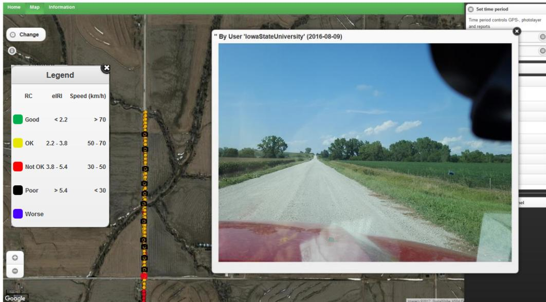
**Figure 4.8. Visualization of the Roadroid roughness test data collected on the L66 test sections on August 9, 2016**
