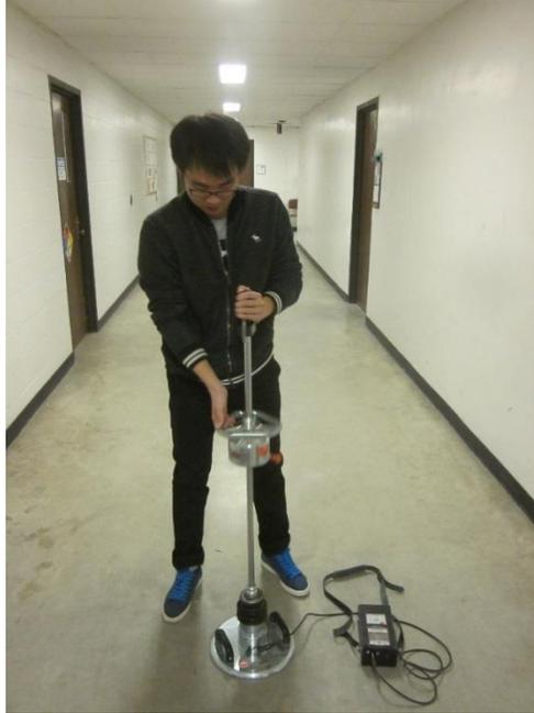
**Figure 4.6. Zorn Model ZFG 3000 LWD used in this study**
