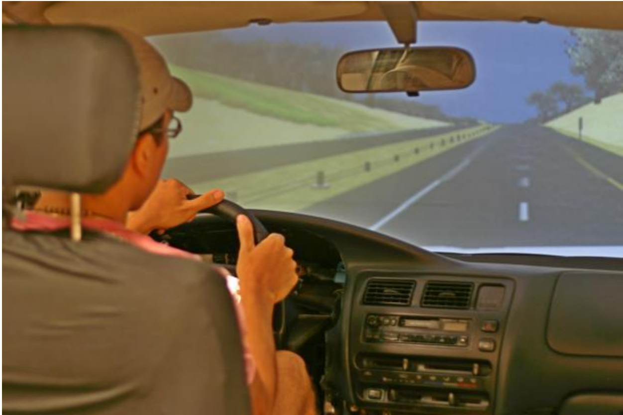
Figure 23. ZouSim driving simulator
