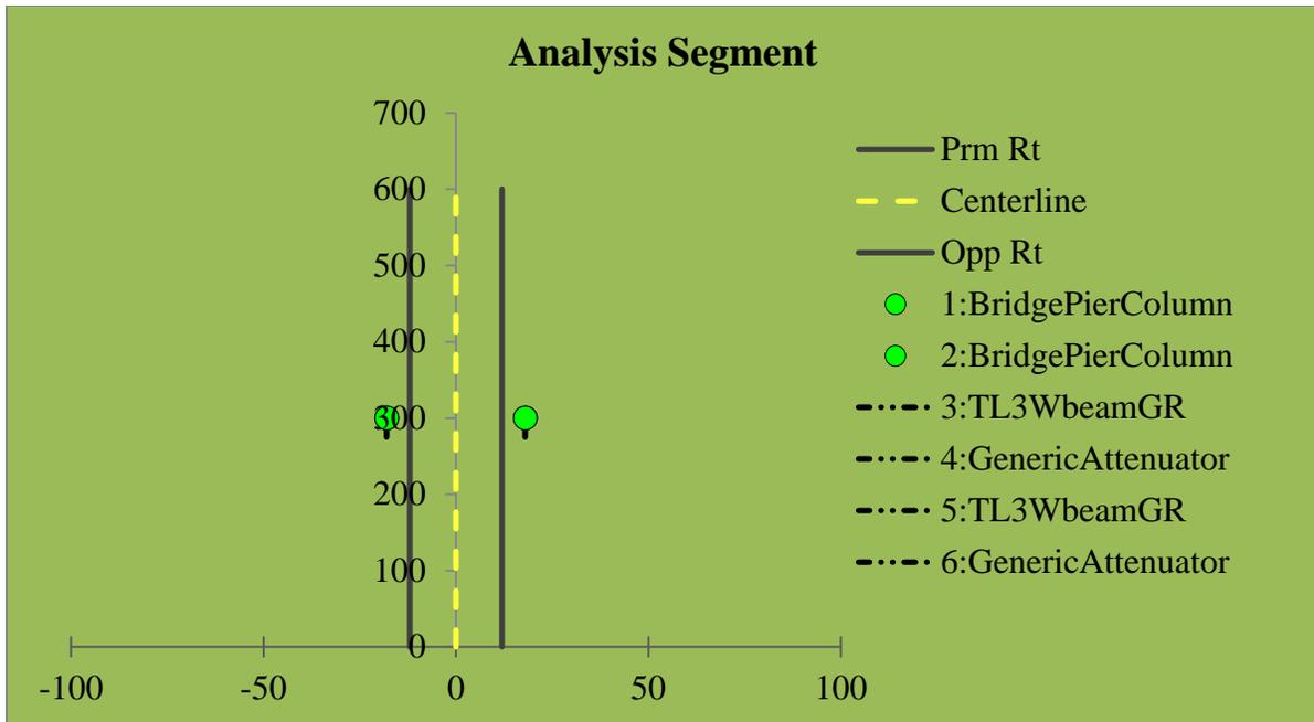
Figure 32. Hazard placement configuration on two-lane undivided highways
