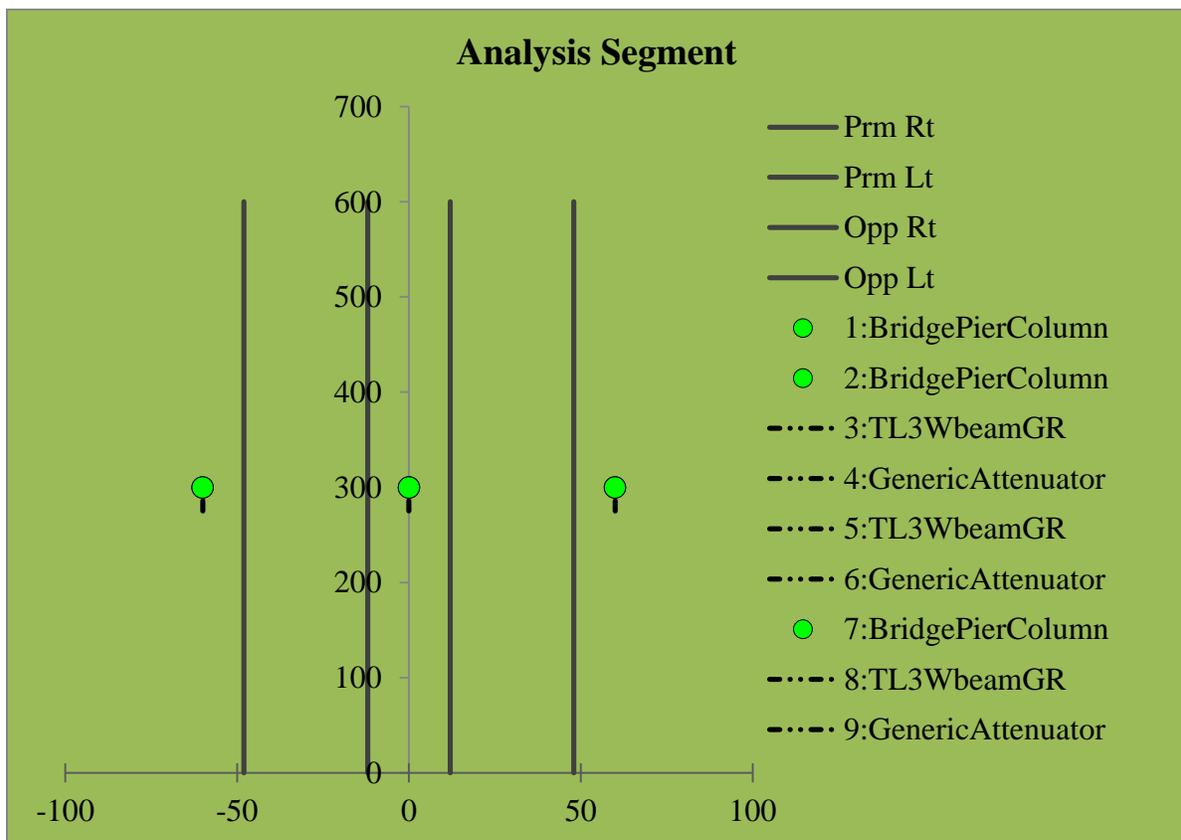
Figure 33. Hazard placement configuration on four-lane divided highways
