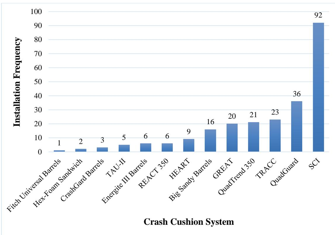
**Figure 4. Installation frequency of crash cushion systems**
