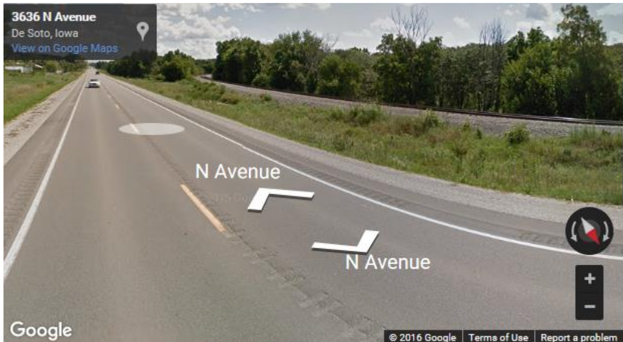
Figure 2. Right continuous with left intermittent
