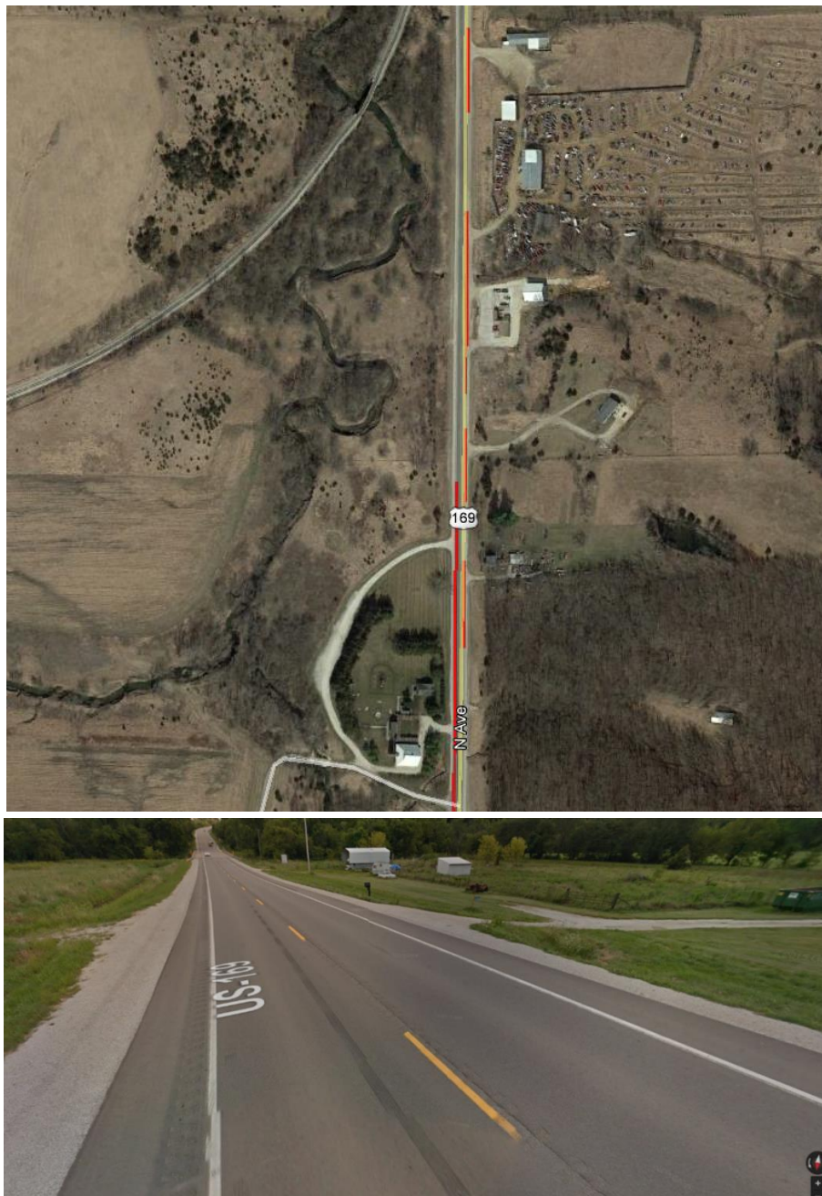
Figure 5. Rumble strip installation with gaps at driveways
