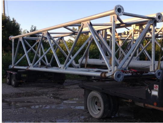
Figure 3.1 Preparation of transported truss for short-term monitoring.
