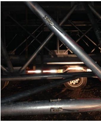
Figure 3.1 Preparation of transported truss for short-term monitoring.
