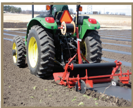
Bedforming, drip tape unspooling, and mulch laying all in one operation.
