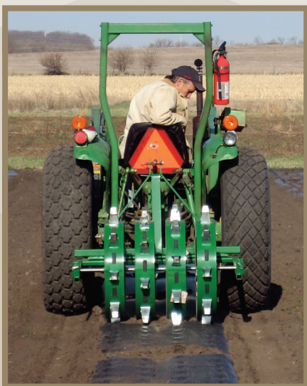
Water wheel marker perforating plastic mulch for seedling plugs.
