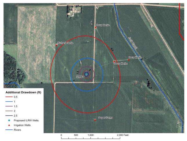
**Figure 13.** Simulated drawdown map for ILRW north wellfield (Well 6) for normal rainfall conditions (8.5 inches of recharge).
