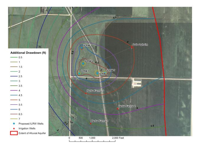
**Figure 16.** Simulated drawdown map for ILRW south wellfield (wells 1 through 5) for a moderate drought (6 inches of recharge).
