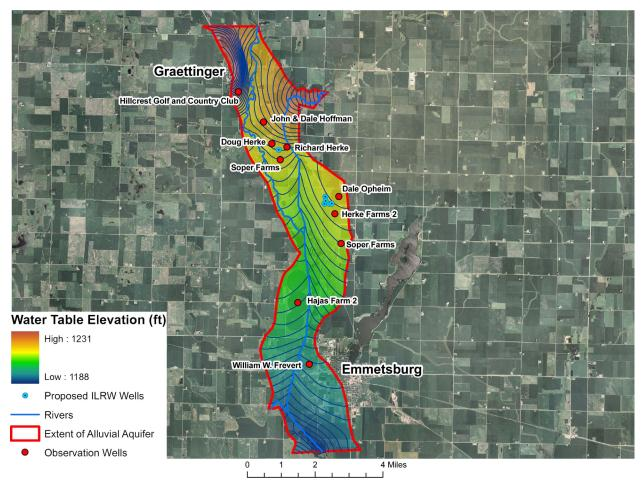
Figure 8. Simulated water table elevation map for non-pumping conditions.
