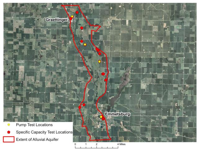
Figure 6. Distribution of specific capacity and pump tests in study area.
