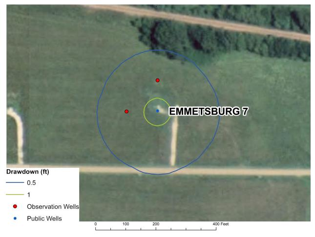
Figure 10. Emmetsburg Well 7 pump test simulation results.
