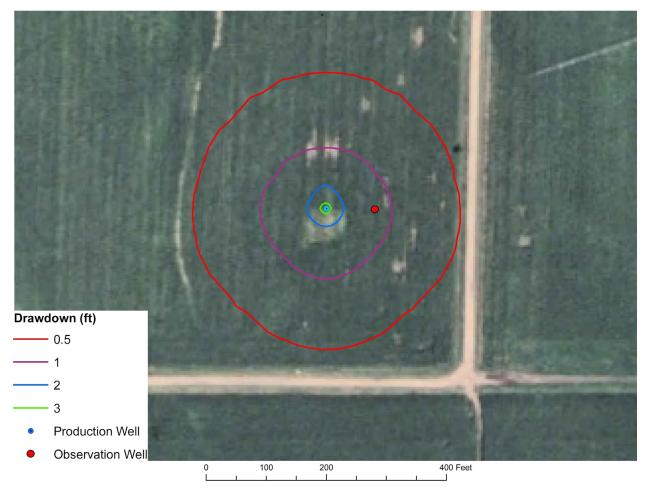
Figure 11. ILRW Test Well P-2B pump test simulation results.
