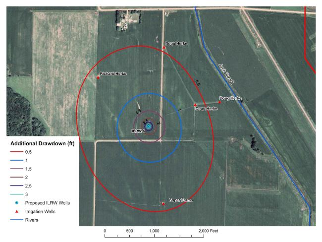
Figure 17. Simulated drawdown map for ILRW north wellfield (Well 6) for a severe drought (4 inches of recharge).
