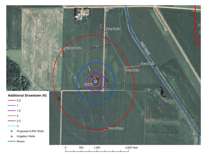
Figure 15. Simulated drawdown map for ILRW north wellfield (Well 6) for a moderate drought (6 inches of recharge).
