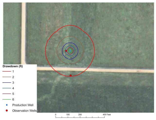
Figure 12. ILRW Test Well P-13A pump test simulation results.
