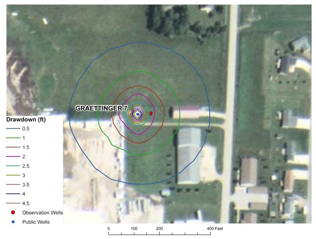
Figure 9. Graettinger Well 7 pump test simulation results.
