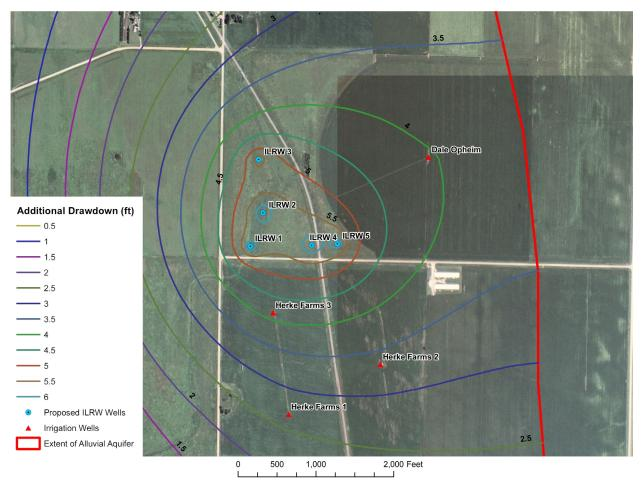
Figure 14. Simulated drawdown map for ILRW south wellfield (wells 1 through 5) for normal rainfall conditions (8.5 inches of recharge).
