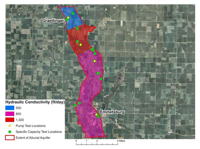
**Figure 7.** Horizontal hydraulic conductivity distribution within active model area based on data found in tables 5 and 6.
