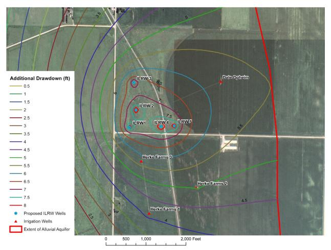
**Figure 18.** Simulated drawdown map for ILRW south wellfield (wells 1 through 5) for a severe drought (4 inches of recharge).
