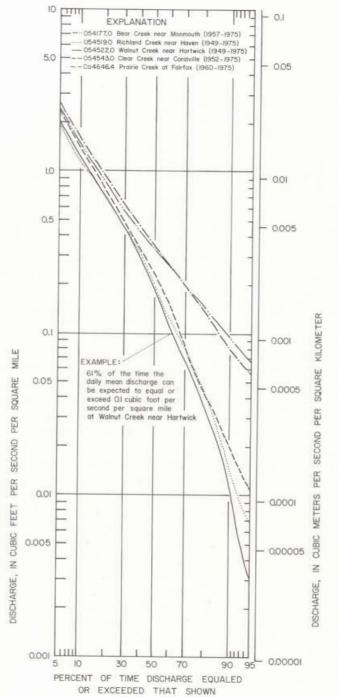
Figure 15.—Flow-duration curves for five east-central Iowa streams
