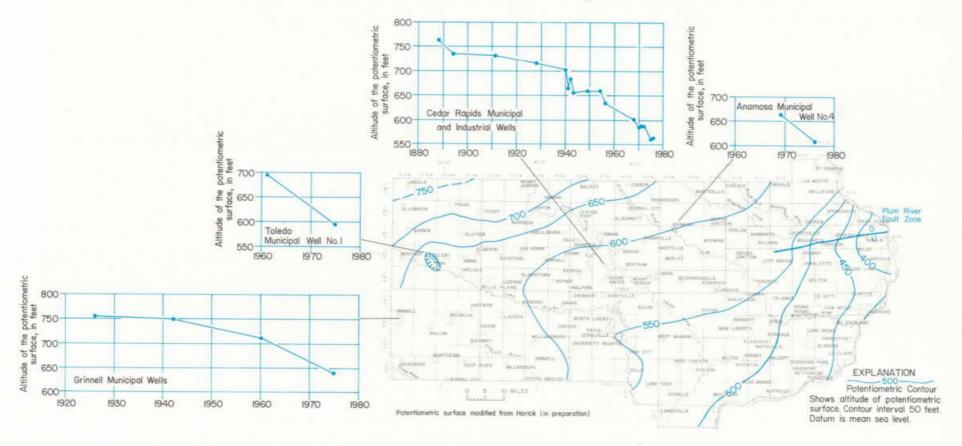
Figure 47.—Potentiometric surface of the Cambrian-Ordovician aquifer in 1975-76, and hydrographs for selected pumping centers
