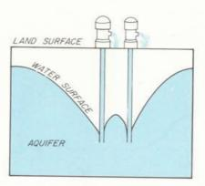
Figure 41.—Drawdown cones around pumping wells
