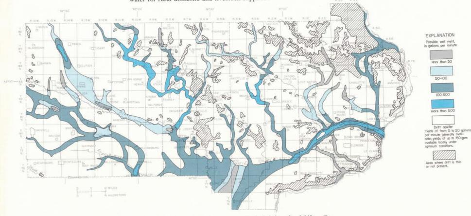
Figure 49.—Possible yields to individual wells; buried-channel and drift aquifers
