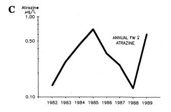
Figure 10. Summary of annual A) groundwater discharge, and B) flow-weighted mean NO<sub>3</sub> and C) atrazine concentrations from Big Spring groundwater.
