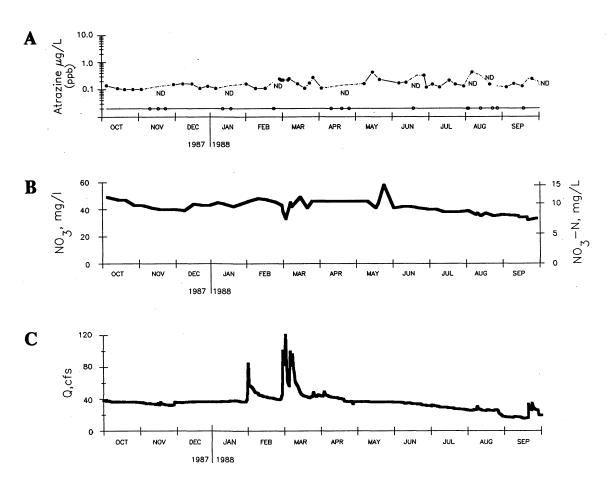
Figure 3. A) Atrazine and B) nitrate concentrations, and C) groundwater discharge at Big Spring for WY 1988.
