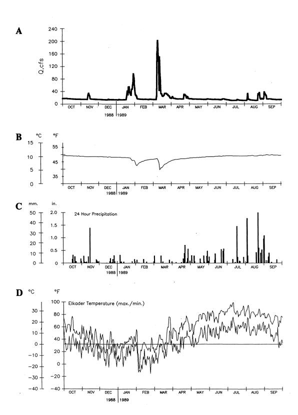
Figure 6. A) Groundwater discharge, B) groundwater temperature, and C) daily precipitation for the Big Spring basin, and D) maximum-minimum temperatures for Elkader, IA (Iowa Dept. of Ag. and Land Stewardship, State Climatology Office), for WY 1989.
