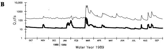
Figure 8. A) Nitrate concentrations and B) discharge hydrographs for Big Spring (bold lines) and the Turkey River (lighter lines) at Garber for WY 1989; (Turkey River discharge data from U.S.G.S., W.R.D., IA Dist.).
