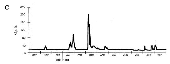
Figure 7. A) Atrazine and B) nitrate concentrations, and C) groundwater discharge at Big Spring for WY 1989.
