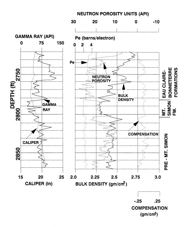
**Figure 1.** Segment of the Schlumberger Litho-Density/Compensated Neutron/Gamma Ray Log between 2720 and 2870 feet showing interpreted upper and lower Mt. Simon Formation contacts in the Eischeid drillhole.
