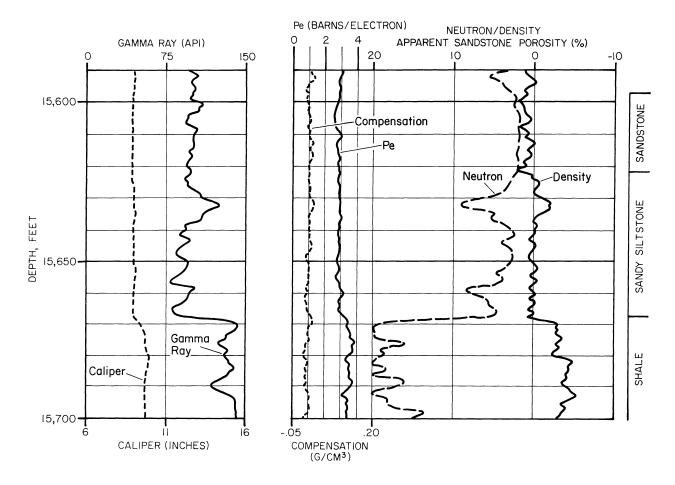
Figure 1. Log responses typical of the clastic sequence in the lower part of Eischeid #1 well. Pe is photoelectric-absorption cross-section. Sandstone intervals are selected on basis of thickness equaling 4 ft (1.2 m) or more, minimal borehole rugosity as shown by caliper and density-compensation traces, Pe less than 3.0, and close agreement of neutron-porosity and density-porosity traces.
