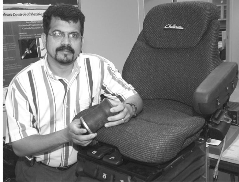
*Atul Kelkar holds a key component of a new pneumatic seat suspension system made for construction and agricultural equipment. Kelkar, chief technology officer for Vibroacoustic Solutions, Inc., and an Iowa State professor of mechanical engineering, says the system offers many advantages over those currently in use.*
