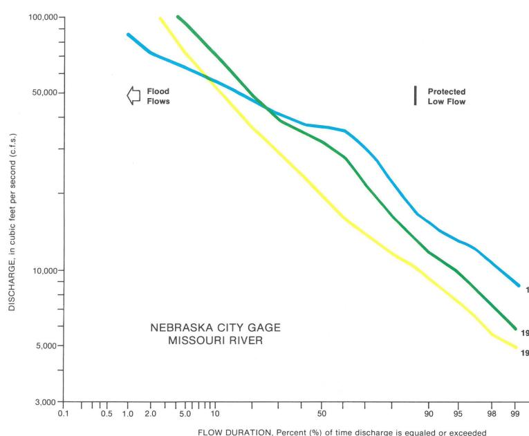
Figure 1. Flow duration curves for the Missouri River, prepared from daily discharge data from the Nebraska City gaging station. Three curves are shown; 1. For the period 1931-1937 when the river was in a natural flow condition; 2. 1938-1957, when the flow was partially regulated; and 3. 1958-1976 when the flow of the river was highly regulated by dams (data, in part, from Lara, in press).
