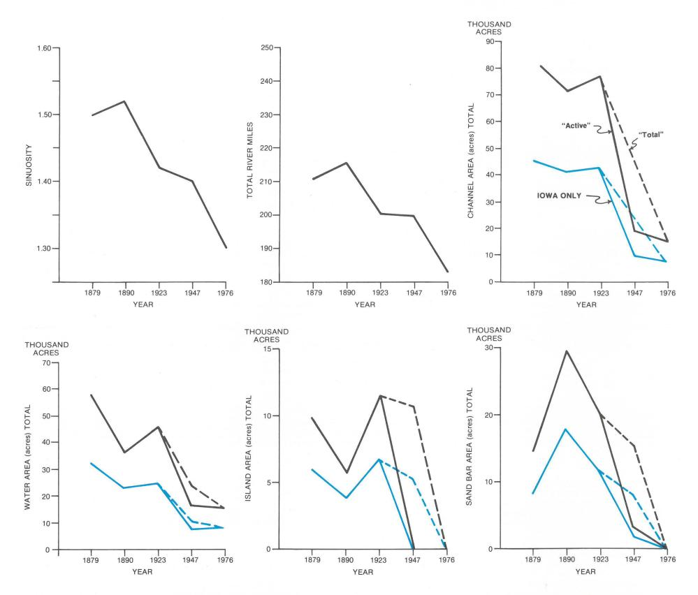
Figure 5. Summary graphs showing changes in the Missouri River channel features adjacent to Iowa, 1879-1976. From 1923 to 1976 the dashed and solid lines show "Active" and "Total" channel categories for 1947 (as defined in Table 4). The Iower blue line shows the trends for the Iowa portion alone.
