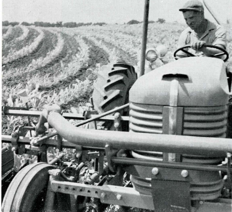
Fig. 7. Furrows and wheel tracks on the contour will hold and store rainfall.
