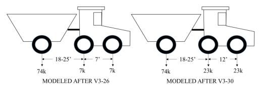
Figure 11. Three-axle controlling vehicles
