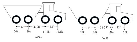
Figure 45. Posting AV vehicles, AV4a and AV4b
