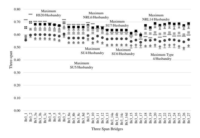
Figure 24. Moment ratios for rating and posting husbandry vehicles for three-span bridges
