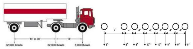
V = Variable drive axle spacing = 6 ft 0 in. to 14 ft 0 in., and use spacing that produces maximum load effects. Neglected axles that do not contribute to the maximum load effect under consideration. Maximum GVW = 80 kips. Axle gage width = 6 ft 0 in.
