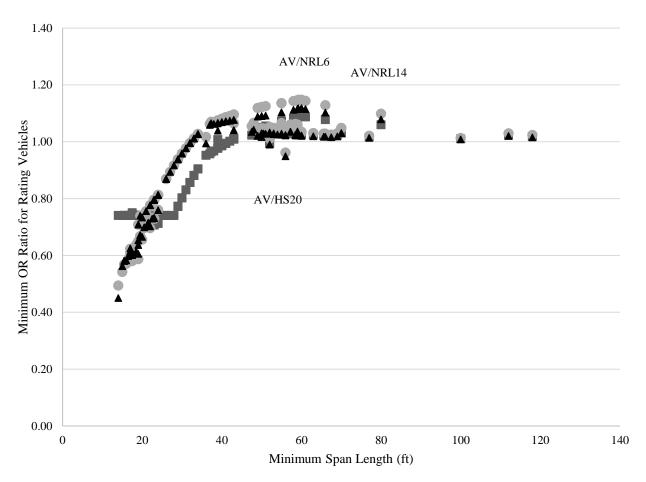
Figure 41. Minimum AV OR ratio versus minimum span length – rating vehicles
