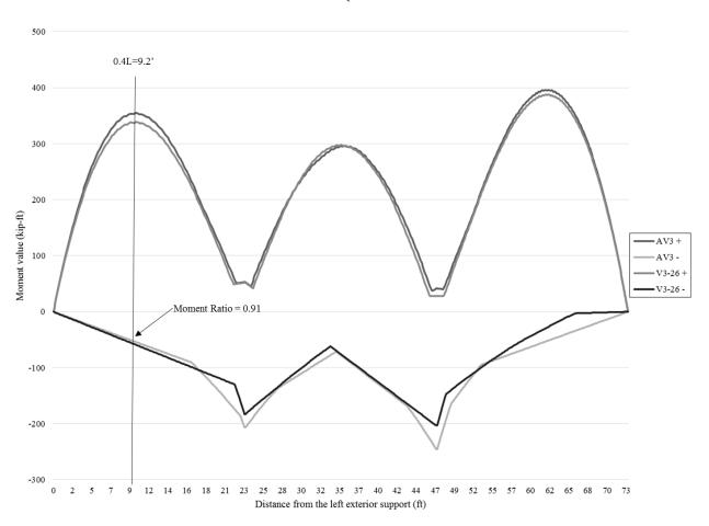
Figure 21. Bridge3\_16 moment envelopes for AV3 and V3-26
