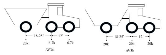
Figure 44. Posting AV vehicles, AV3a and AV3b
