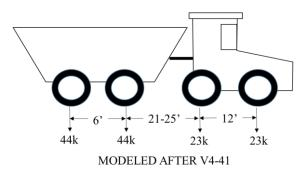
Figure 12. Four-axle controlling vehicle
