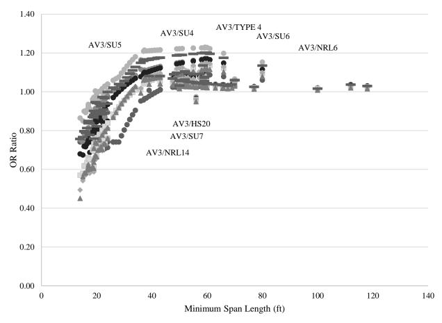
Figure 38. AV3 ratio versus minimum span length
