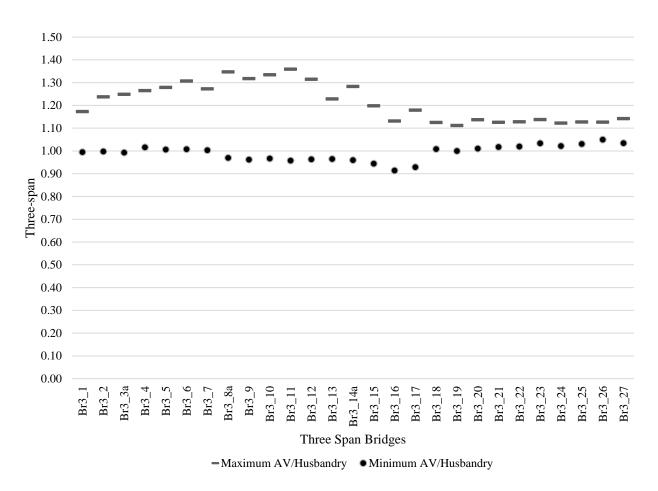
Figure 19. Moment ratio plot for AV/husbandry for three-span bridges
