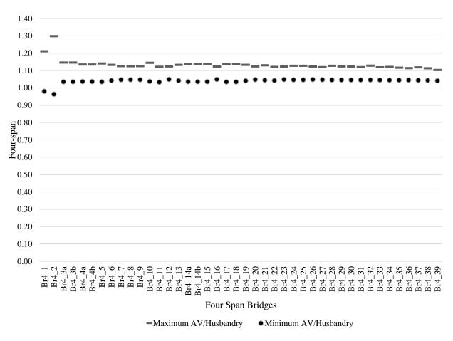
Figure 20. Moment ratio plot for AV/husbandry for four-span bridges
