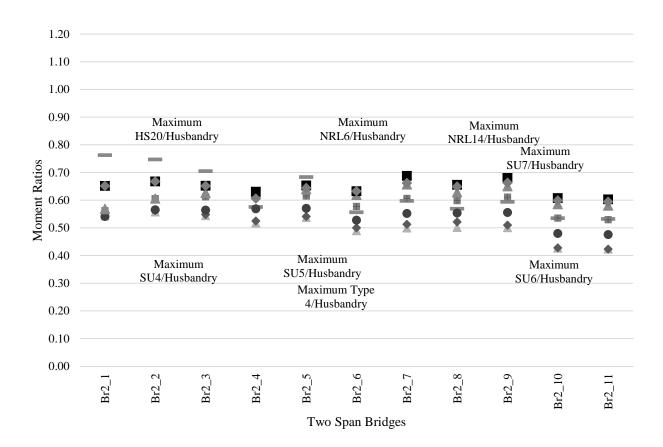
Figure 23. Moment ratios for rating and posting husbandry vehicles for two-span bridges
