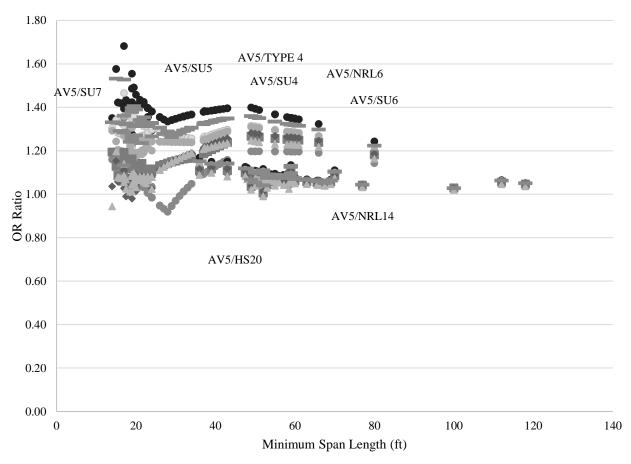
Figure 40. AV5 ratio versus minimum span length
