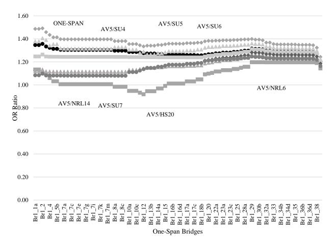
Figure 28. AV5 ratios for one-span bridges
