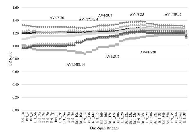
Figure 27. AV4 ratios for one-span bridges
