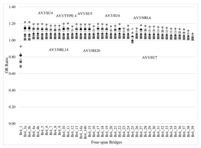
Figure 35. AV3 ratios for four-span bridges
