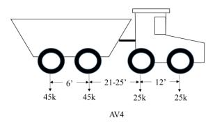
Figure 15. Four-axle generic agricultural rating vehicle, AV4
