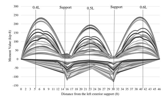
Figure 6. Three-span bridge, Bridge3\_1, moment envelopes and critical locations for 121 husbandry vehicles
