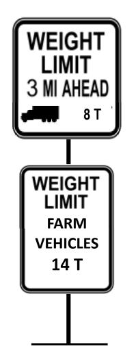
Figure 48. Posting sign for a longer bridge
