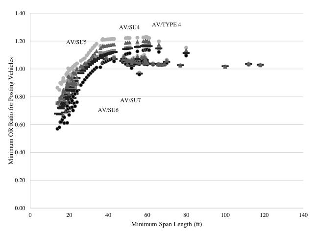
Figure 42. Minimum AV OR ratio versus minimum span length – posting vehicles
