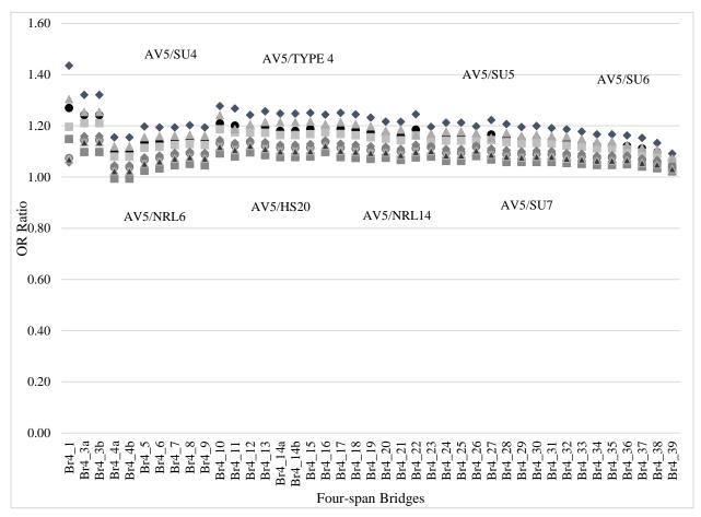
Figure 37. AV5 ratios for four-span bridges
