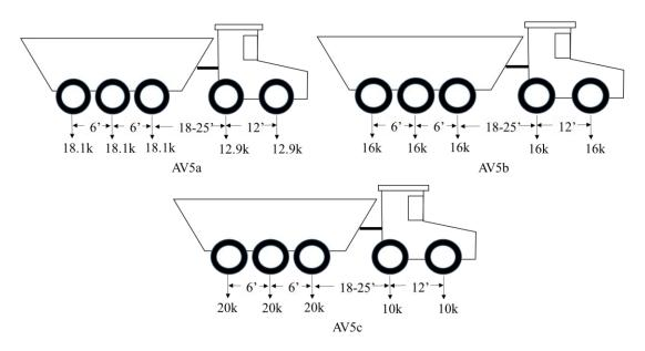
Figure 46. Posting AV vehicles, AV5a, AV5b, and AV5c
