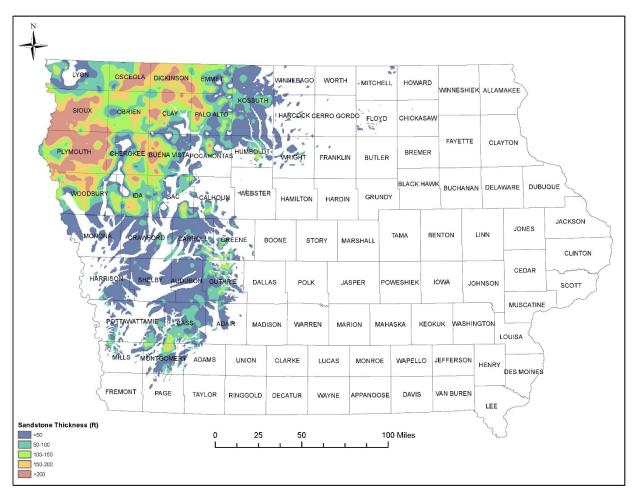
**Figure 9.** Lower Dakota aquifer isopach map in Iowa generated by combining Figure 5 with work completed by Gannon et al. (2008).
