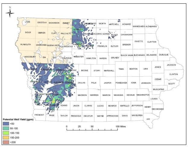
**Figure 8.** Estimated potential well yields in the Lower Dakota aquifer within the study area based on transmissivity, specific capacity data, and available drawdown.
