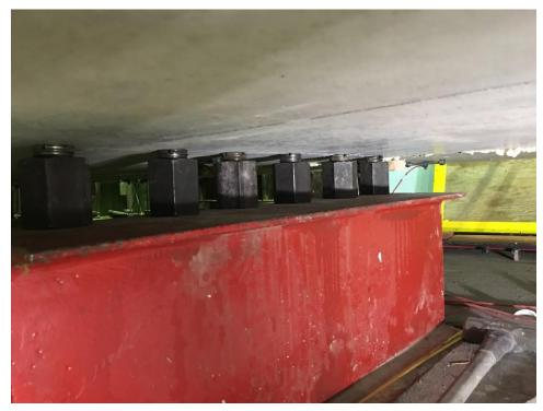
Figure 36. Restraints under one beam
