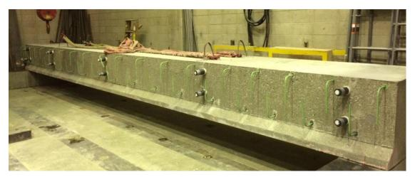
Figure 23. Side of the box girder with hook bars installed
