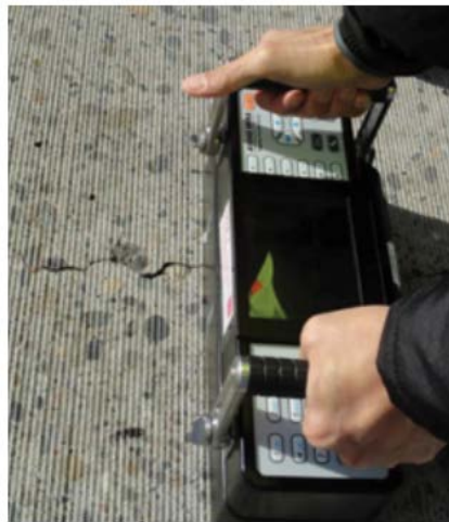
Figure 88. MIRA ultrasonic shear-wave tomography device
