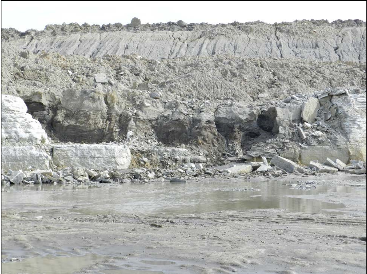
Figure 10. Photo of the working face looking northeast from inside the US Gypsum Flintkote quarry. Note the thickness of the glacial sediment package overlying the gypsum and the irregular bedrock surface. (Photo taken by Ryan J. Clark on 3/18/2014 and used with permission by the US Gypsum Company.)
