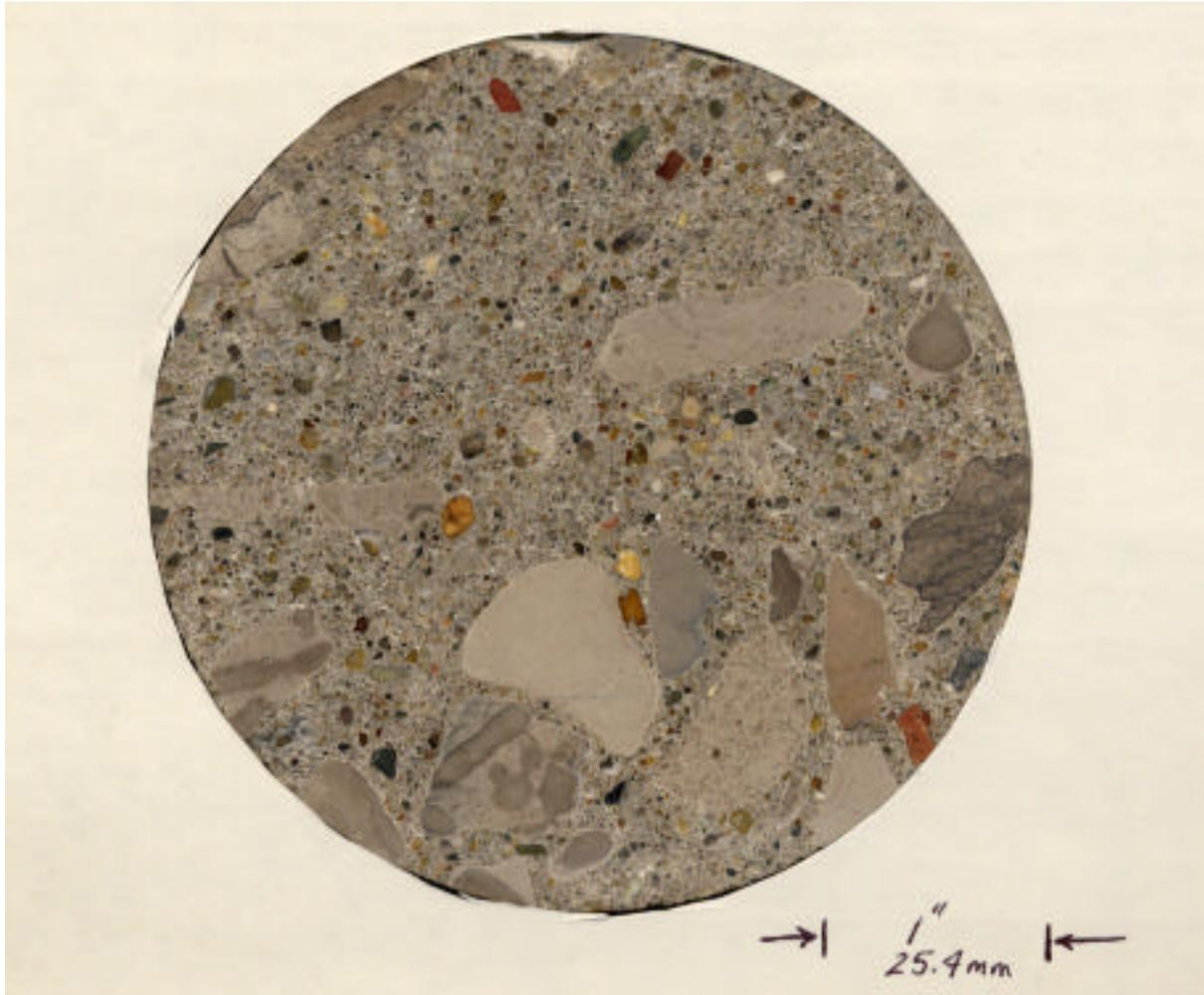
**FIGURE 8** Illustration of segregation in a core extracted from I-80 in Iowa county.
