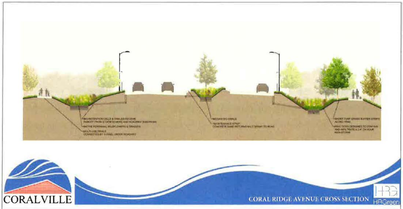
Figure 2: A cross section of bio cells surrounding Coral Ridge Avenue
