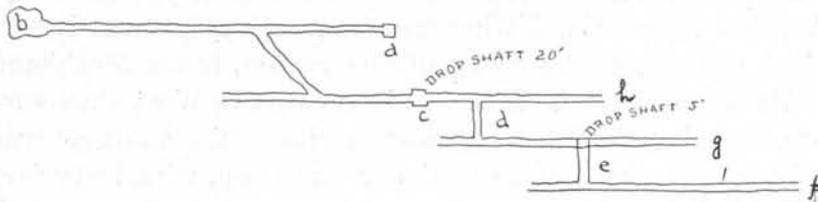
Fig. 91. Ground plan of Kane Bros. mine.
