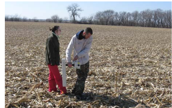
Two types of magnetic gradiometers in use at the Kimball Village site. Above, Bartington 601 dual fluxgate. Below Geoscan Research FM256 fluxgate.
