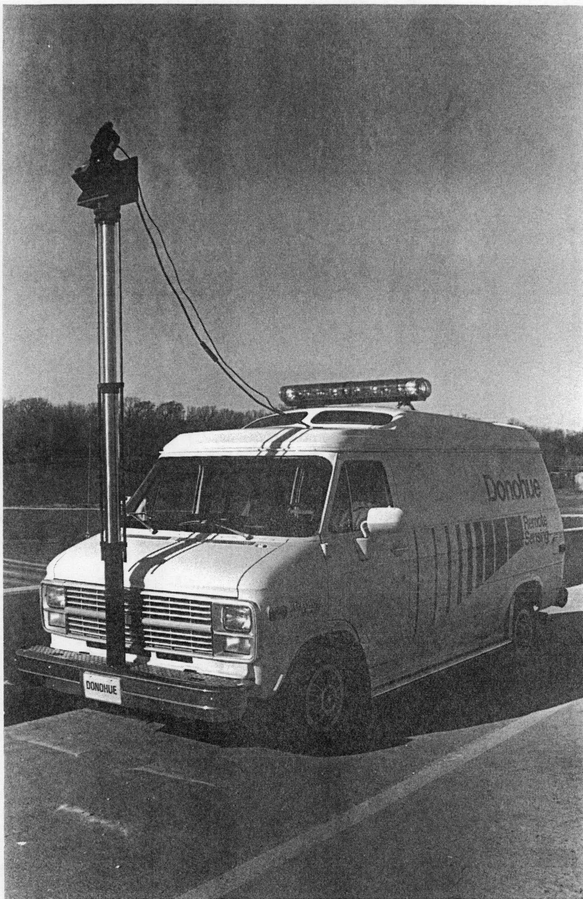
Figure 4 Infrared data collection van
