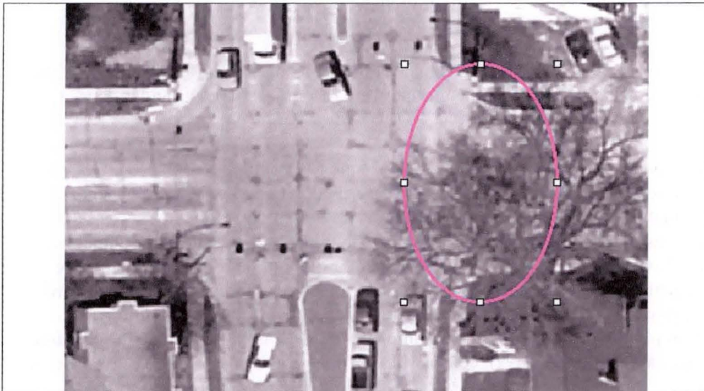
Figure 4-1: Underestimation of signals due to vegetation cover
