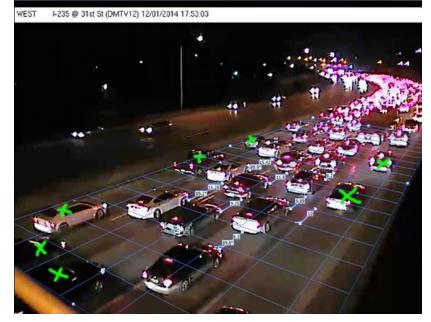
Camera image processed to obtain standstill distance measurements
