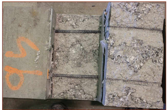
Pull-off test specimen failure at the concrete bond interface showing the failure planes on the substrate concrete surface in the center and the overlay concrete surface on the right
