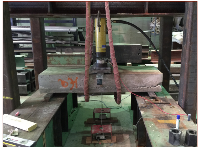
Negative bending flexural test specimen with substrate concrete on top and overlay concrete on the bottom
