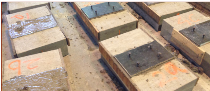
Pull-off test specimens in overlay formwork with studded steel plates pushed into overlay concrete on top
