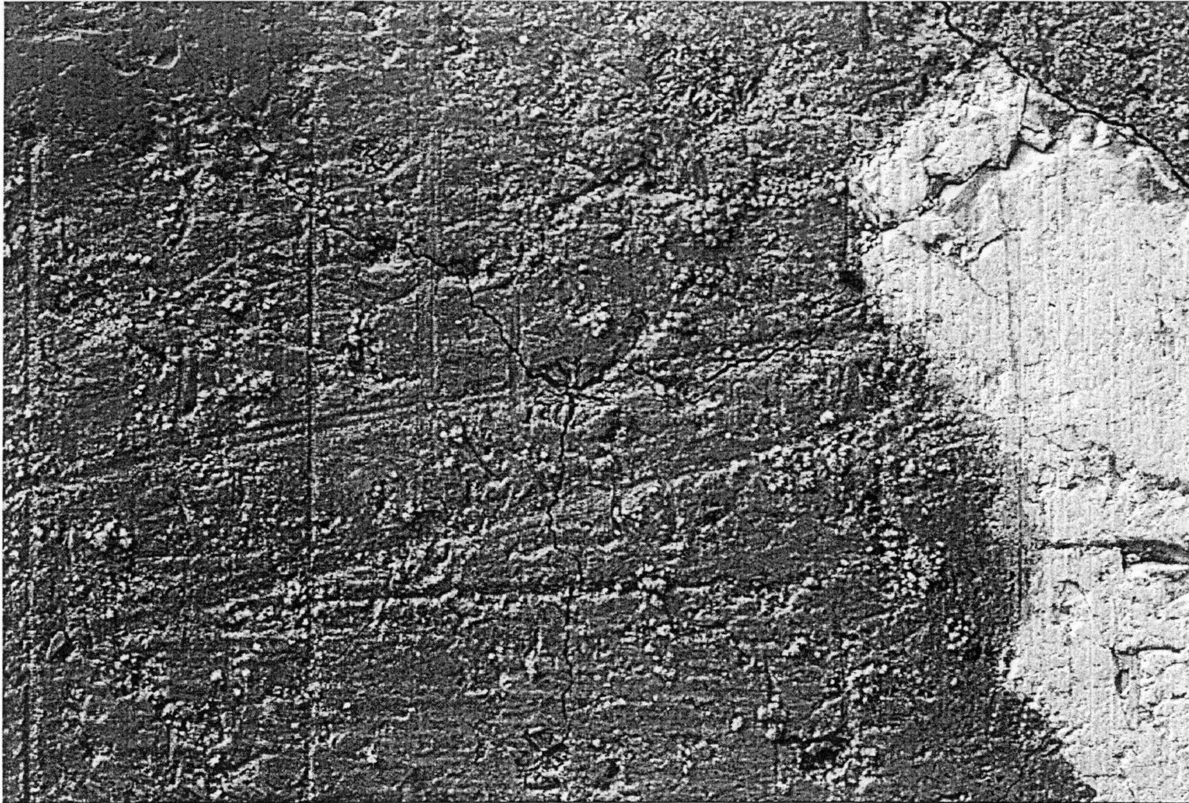
FIGURE 4 A 200X BSE PHOTOMICROGRAPH OF THE PCC AIR VOIDS ON IOWA US 20
