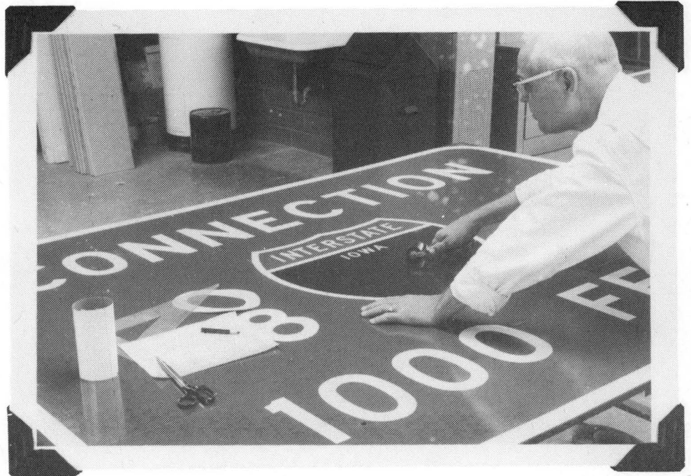
a D.O.T. sign shop worker fabricating a highway sign
