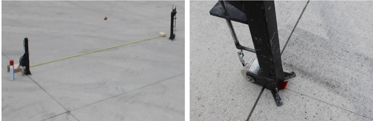
Figure 36. Field test on November 10, 2014: setup overview (left) and clips used in the ends (right)
