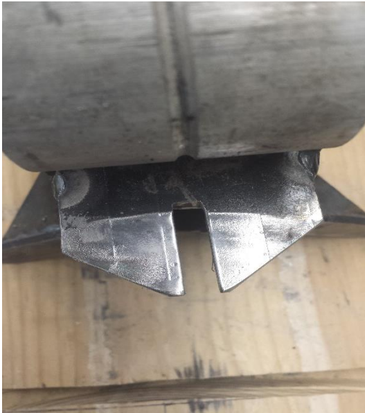
Figure 46. Improvements made for fourth generation of ISU curling and warping measurement device: shorter head of column A (top left), shorter handle of column B (top right), sharp anchor (bottom left), and replaced cord (bottom right)
