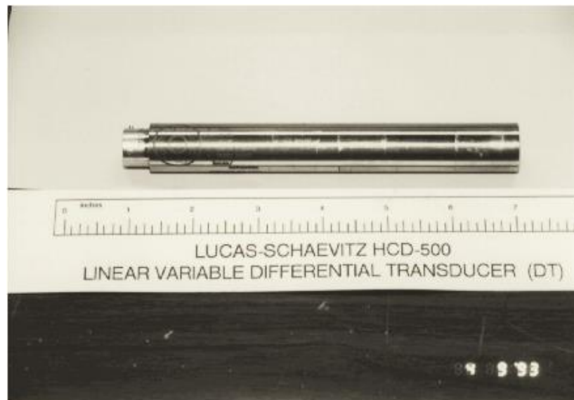
Figure 2. LVDT used for vertical deflection measurement in concrete pavement
