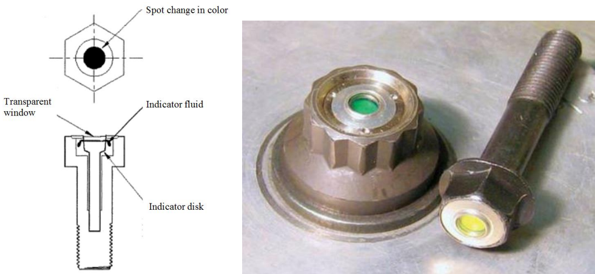
Figure 2-6. Tension-indicating bolt with indicator fluid
