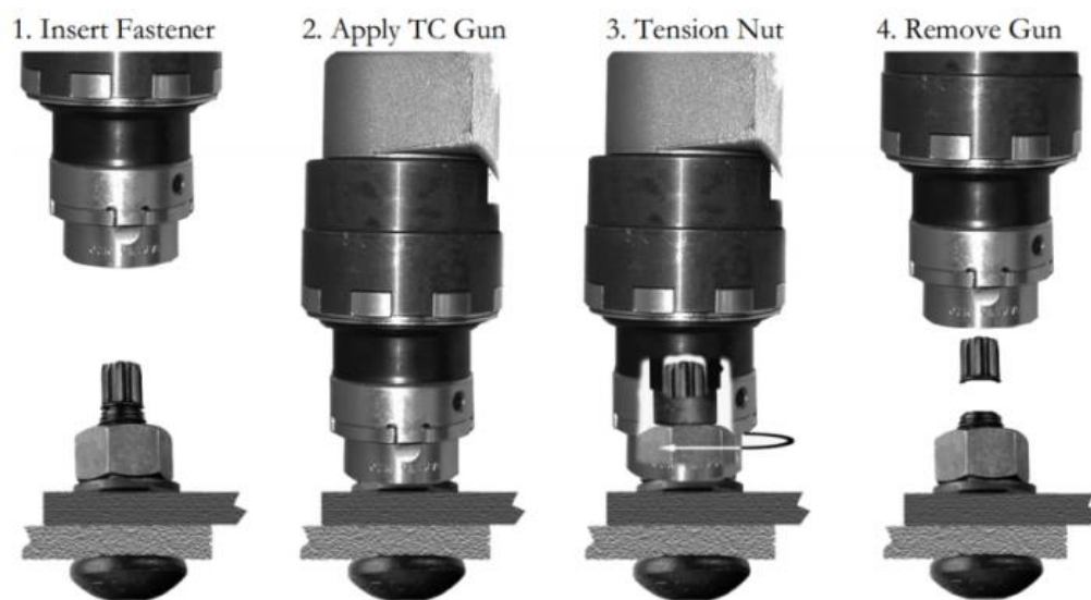
Figure 2-10. Twist-off-type installation procedure
