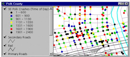
Figure 4: The spatial pattern of accidents by time of day can be easily displayed using the power of a GIS.
