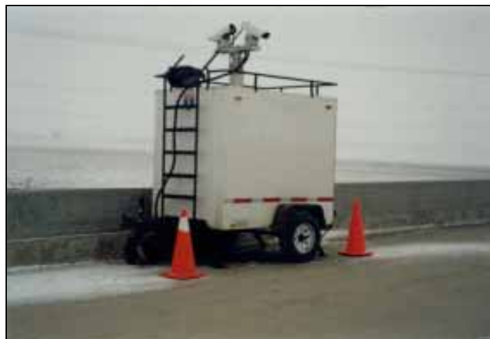
Figure 13. AutoScope video traffic detection system
