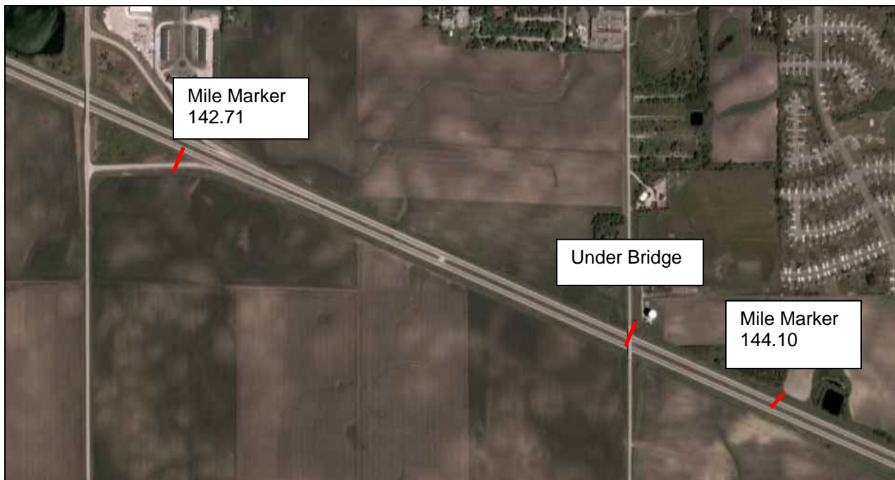
Figure 19. Placement of pneumatic road tubes
