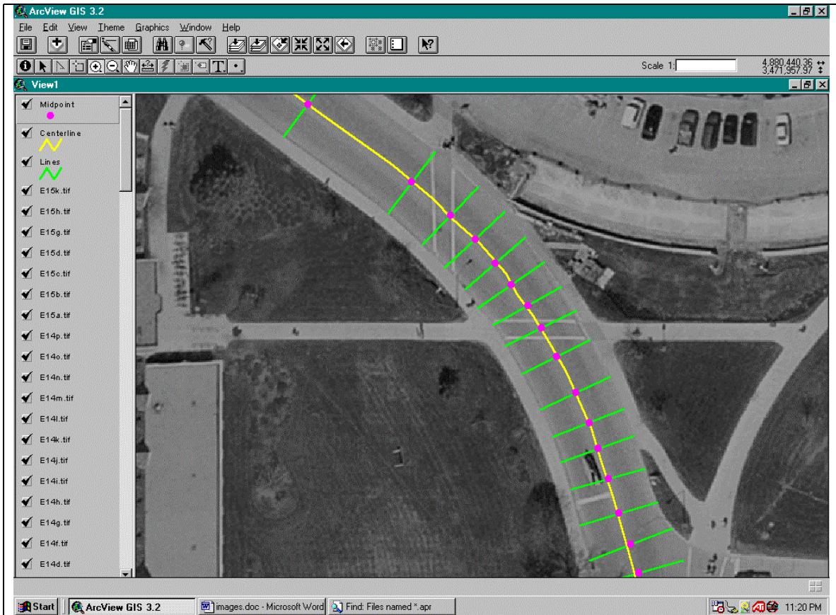
Figure 7. Calculation of Roadway Centerline
