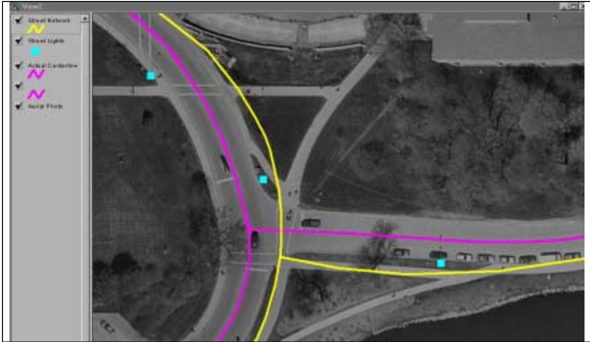
Figure 15. Points Mapped to Wrong Side of Segment (Cartography vs. Centerline)
