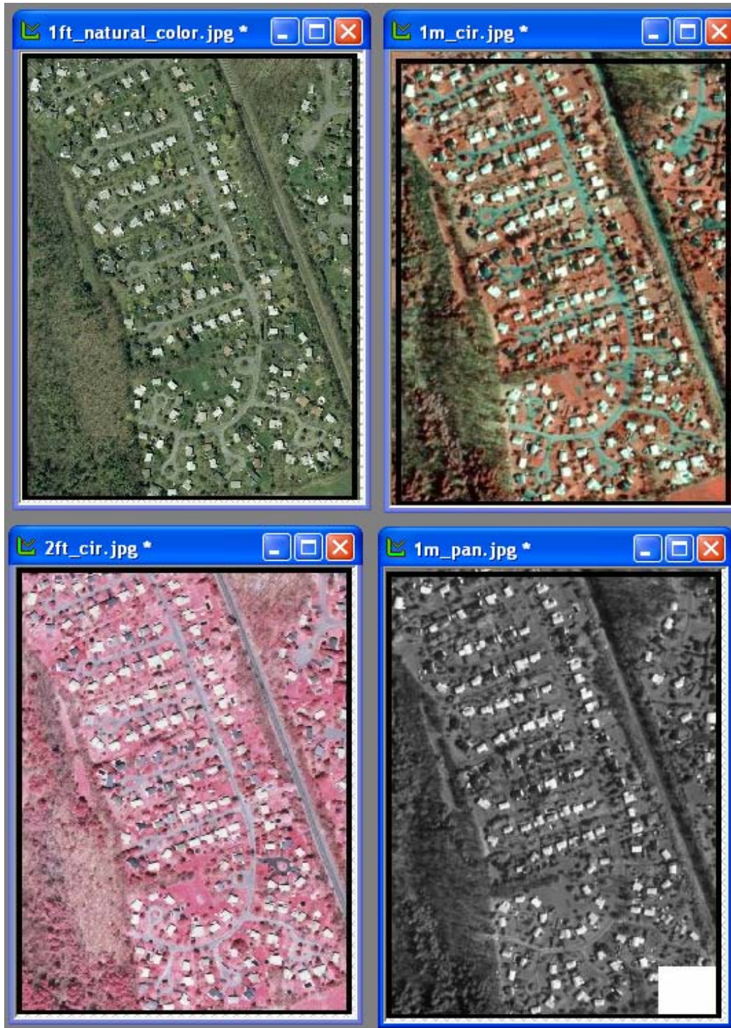
Figure 8. Difference in spectral resolution for one square mile analysis grids
