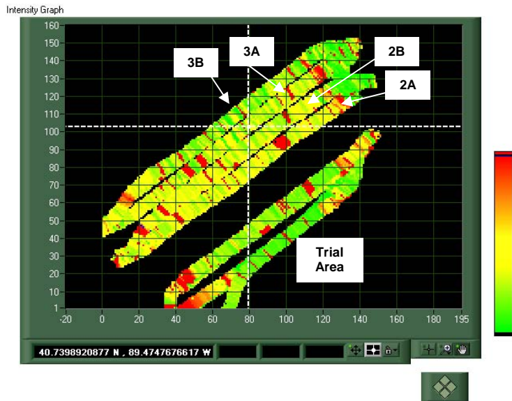
Figure 16. Compaction monitor results for test strips 2 and 3
