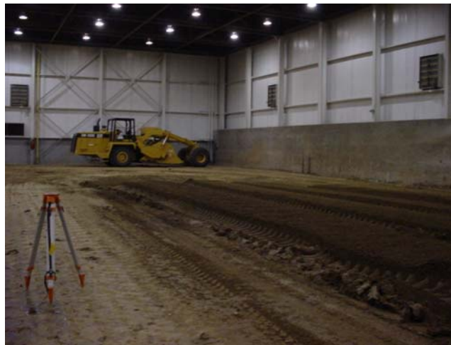
Figure 32. Test strips F and G after tilling with RR350
