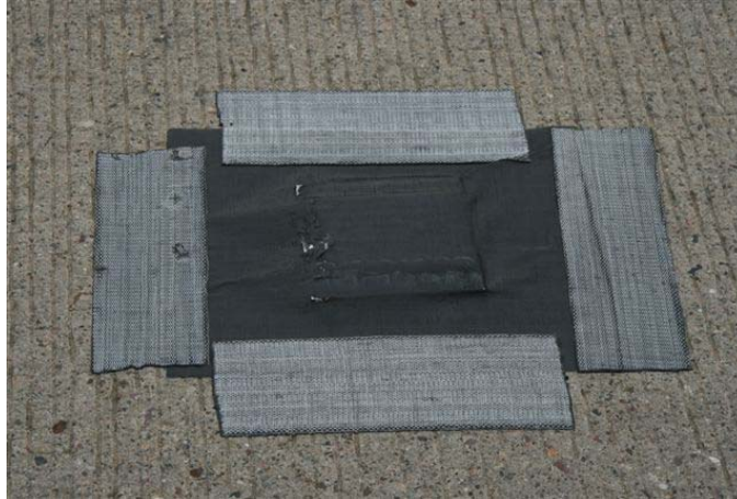
Figure 13. Typical NuMetrics plate counter installation (photo by Brad Grefe, CTRE)
