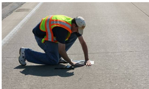
Figure 12. Placing NuMetrics plate counter (photo by Brad Grefe, CTRE)
