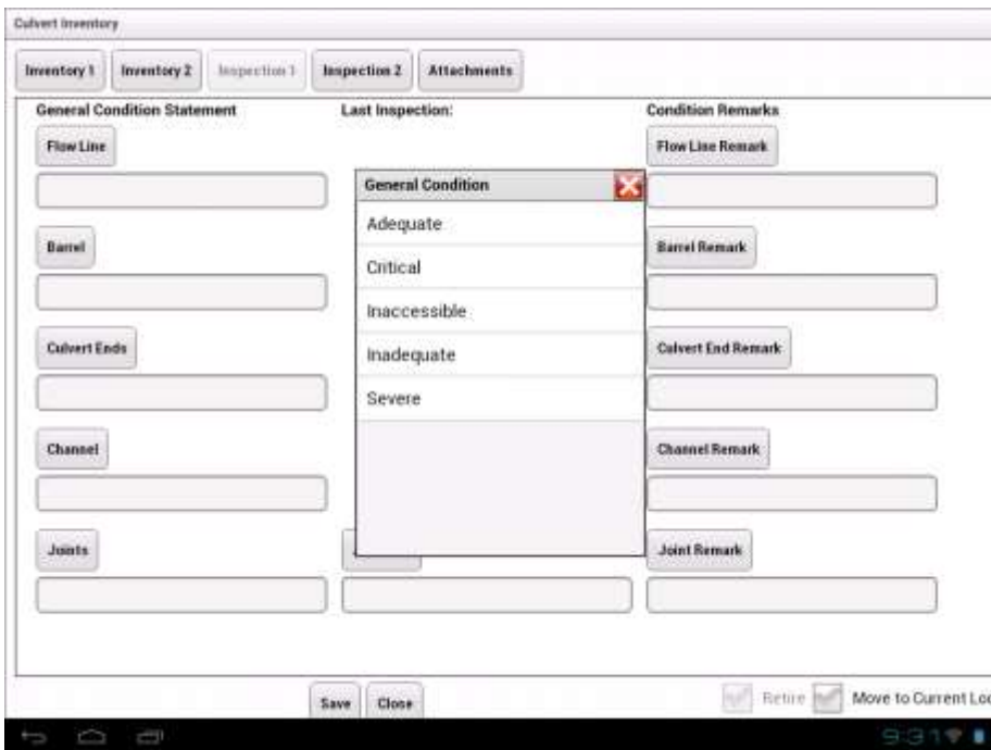
Figure 3 – MAVRIC culvert inspection first screen with a pick list example.
