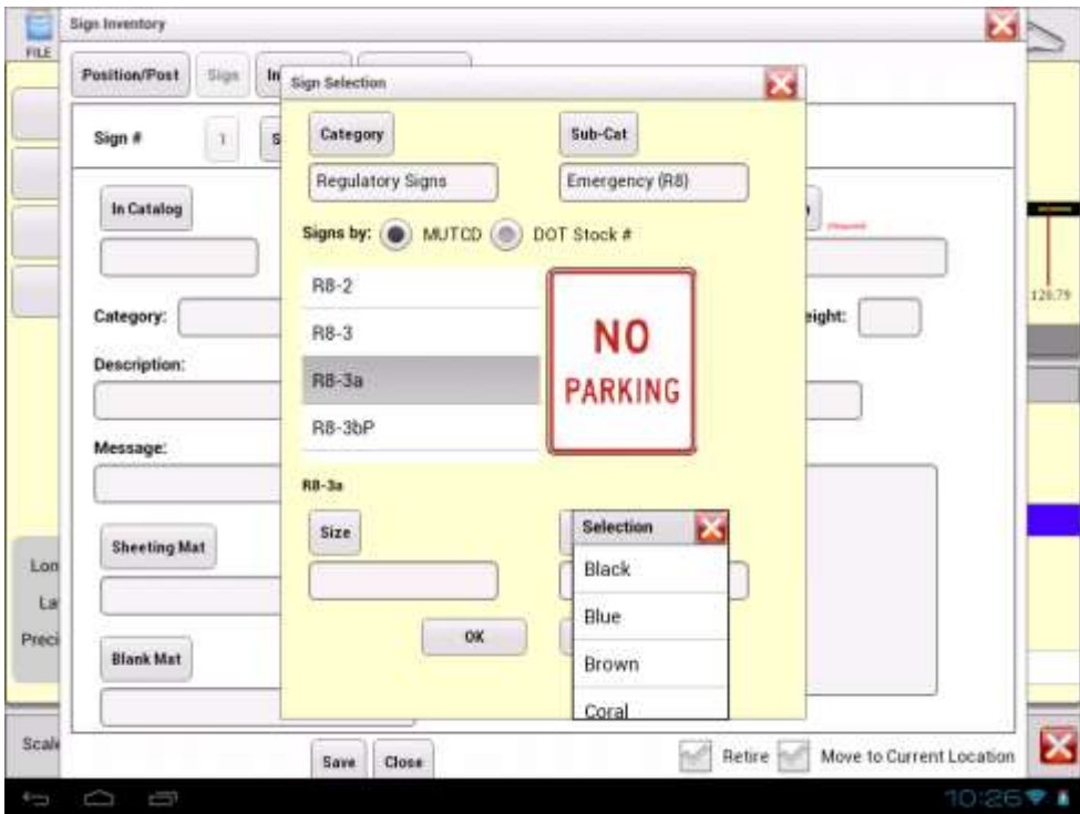
Figure 5 – MAVRIC sign inventory, sign designation screen with images available when assigning a sign type.
